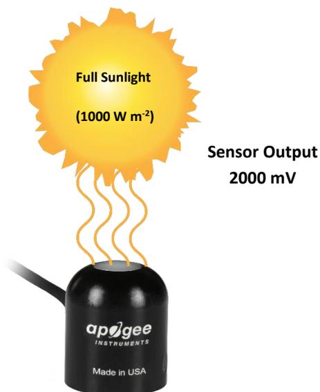
**Serial Number Range 0-10516.** Example of total shortwave radiation measurement with an Apogee SP-212 pyranometer. Full sunlight yields total shortwave radiation on a horizontal plane at the Earth's surface of approximately 1000 W m<sup>-2</sup> s<sup>-1</sup>. This yields an output signal of 2000 mV. The signal is converted to shortwave radiation by multiplying by the calibration factor of 0.5 W m<sup>-2</sup> per mV.
