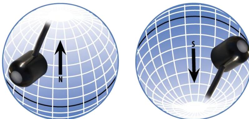
In addition to orienting the cable to point toward the nearest pole, the sensor should also be mounted such that obstructions (e.g., weather station tripod/tower or other instrumentation) do not shade the sensor. **Once mounted, the green cap should be removed from the sensor.** The green cap can be used as a protective covering for the sensor when it is not in use.
